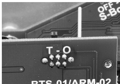
VarioTrack termination activated (position T)
