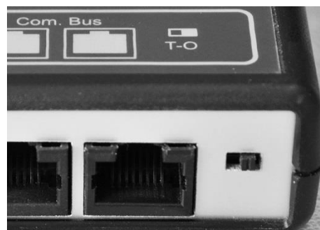
BSP termination deactivated (position O)
