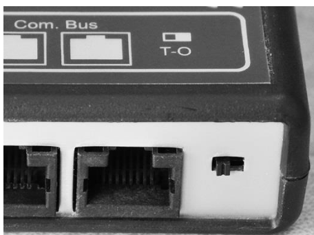
Xcom-232i termination activated (position T)
